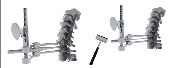
Final impaction can be performed gently with the final impactor. Once the distractor is released, check the correct stability of the cage.
